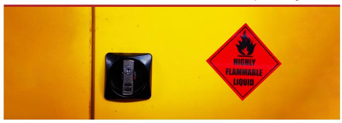
Flammable and combustible liquids are a significant fire-load hazard for any business. To limit the potential for a serious fire event, these liquids should be stored safely and properly. This resource serves to define what a flammable storage cabinet is and how they should be used.
